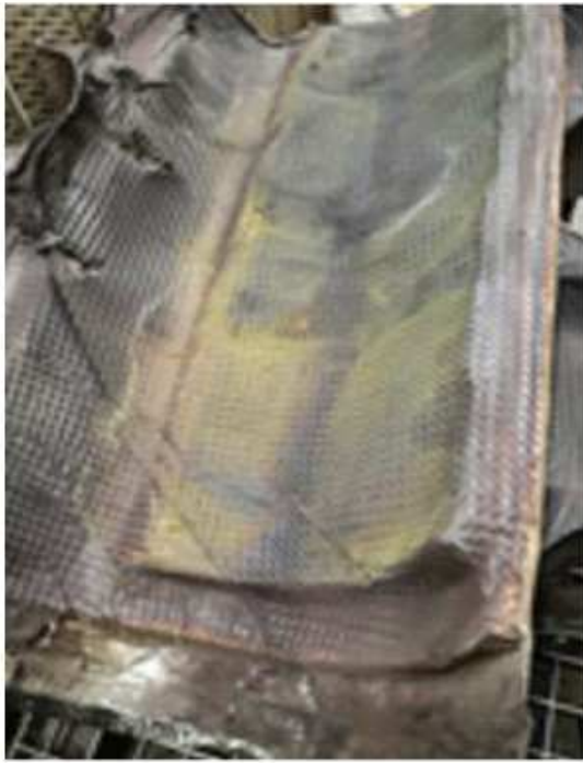
Illustration 1 Exhaust system examples of yellow residual deposits
