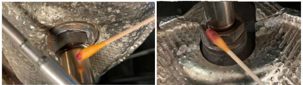
Figure 2: Screwed sensors on insulated exhaust pipe with positive Cr(VI) rapid test
