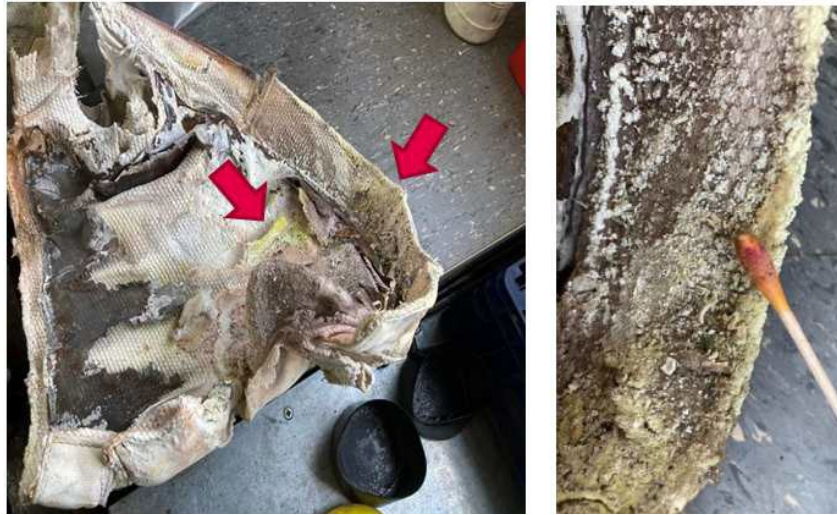
Figure 1: Insulation blanket of an exhaust gas turbocharger with positive Cr(VI) rapid test
