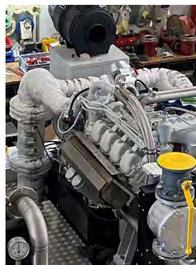
Fig. 70/Fig.71 Exhaust gas pipe CHP insulated calcium-free
