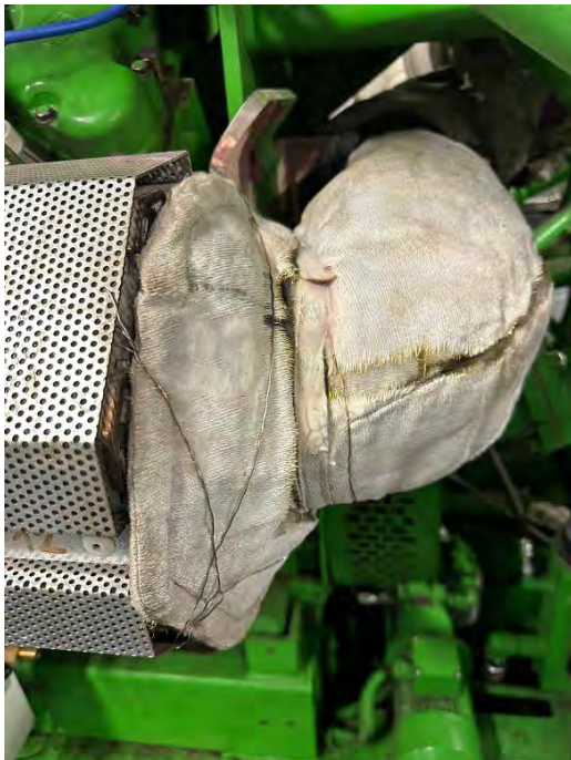
Fig.47: Chromates on the surface of textile insulationsFig.
