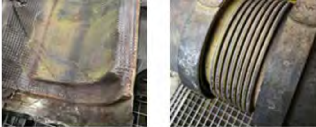
Illustration 1 Exhaust system examples of yellow residual deposits
