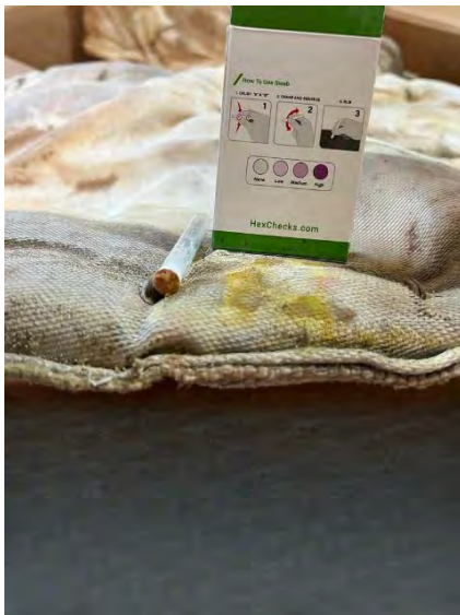
Fig. 60-64: Chromate deposits on insulating mattresses
