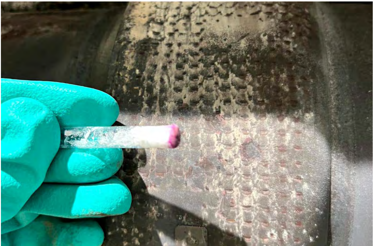
High calcium chromate concentration on almost all hot engine parts of a gas engine (Fig. 44)
